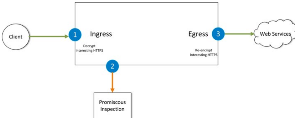
Figure 12: Traffic flow in the BIG-IP solution with cloning
