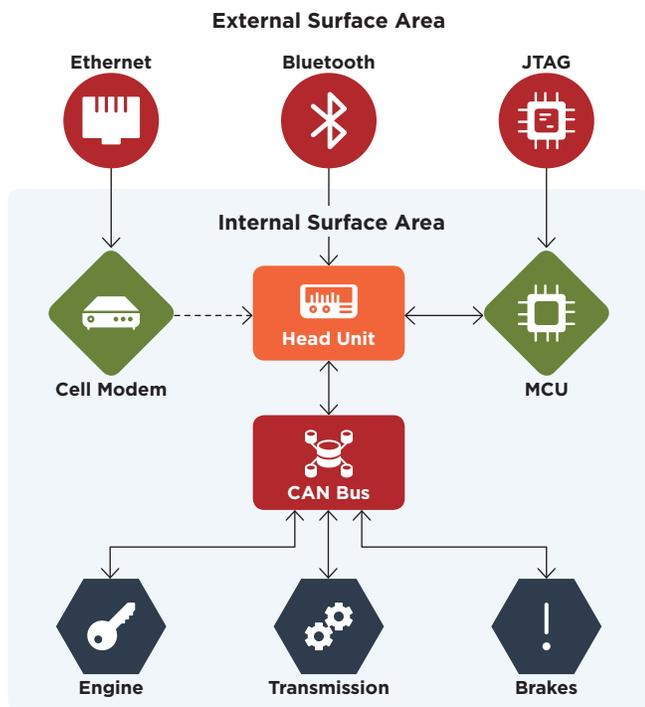
Sample threat model of a connected car.
